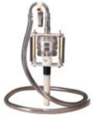
cyclone in the US is the Dorr-Oliver, 10mm nylon cyclone. It was first utilized in US coal mines in the early 1960's, and it continues to be the most commonly used model in the US. It will follow the US ACGIH size distribution curve (50% cut at 4 microns) closely when used at 1.7 LPM. This cyclone is specified in numerous NIOSH and OSHA Test Methods for use with 37mm, 5 micron, PVC,
