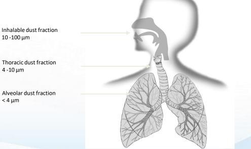
The Respicon system is a simulation of the human breathing tract and measures the three fractions of dust humans are exposed to simultaneously
