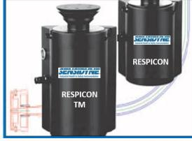
Respicon TM : Combined gravimetric/photometric system
