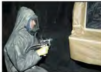
Worker applying spray-on polyurethane truck bed liner. Source: Wikimedia / Creative Commons
