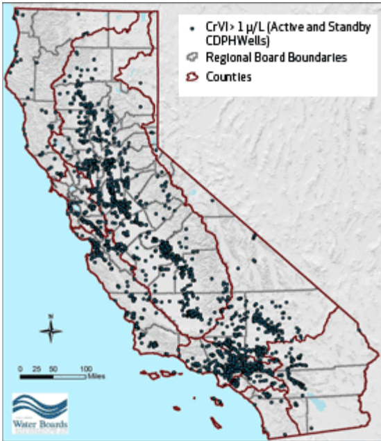
Active and Standby CDPH Wells (3156 Total) with at Least One Detection of Chromium VI > 1 µg/L DLR
