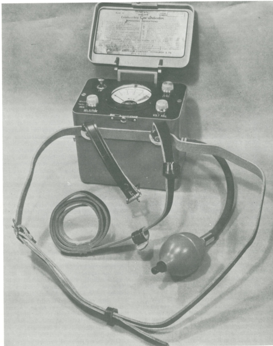
Fig. 1. M-S-A Model 40 Combustible Gas Indicator for Locating Gas and Testing Flammable Gas or Vapor Hazards
