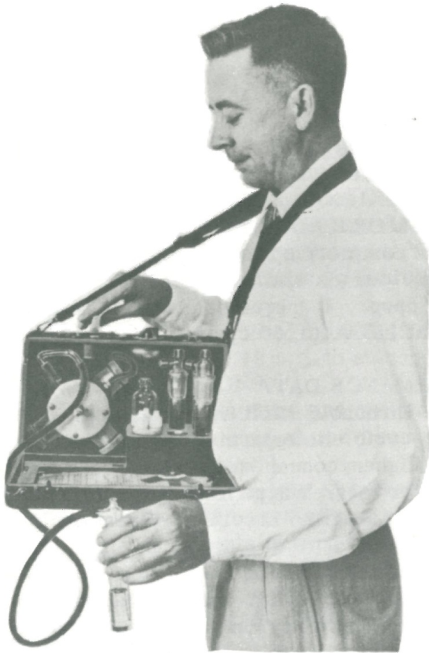
Fig. 1. TDI Detector Kit in Use.
