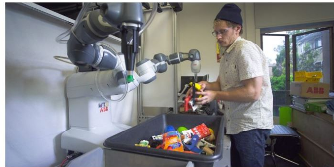
Filling a bin with objects for the Dex-Net 4.0 robot grasping research. Credit: Adriel Olmos, UC Berkeley
