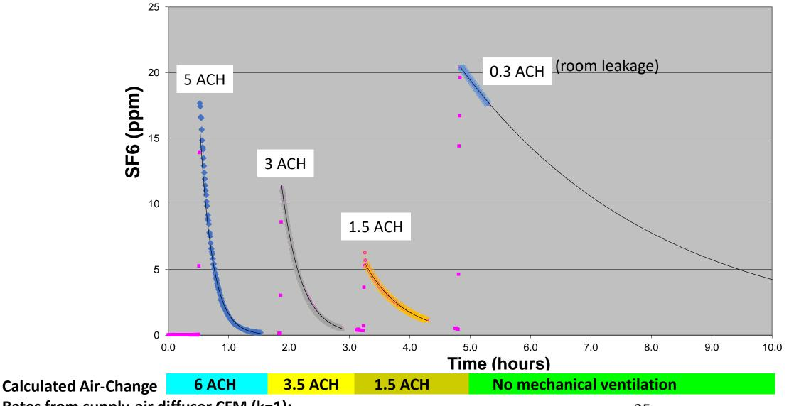
Rates from supply-air diffuser CFM (k=1):
