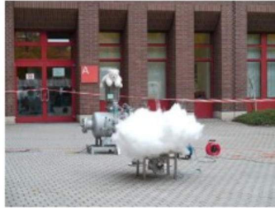
Finely-ground flour is dispersed
