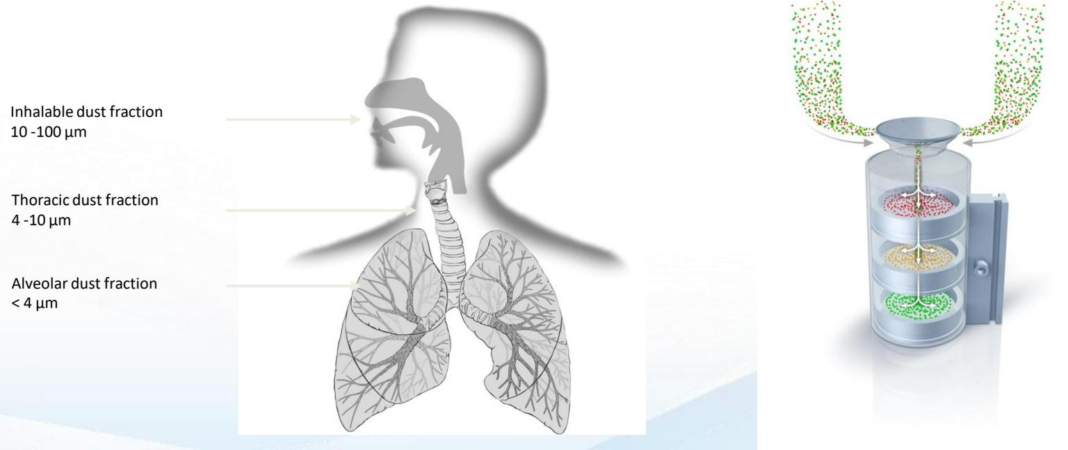
→ The Respicon system is a simulation of the human breathing tract and measures the three fractions of dust humans are exposed to simultaneously
