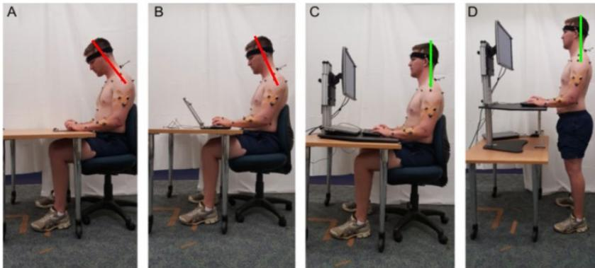
Fig. 1. Device placement for each experimental condition: (A) tablet, (B) laptop, (C) desktop, sitting, and (D) desktop, standing, with retro-reflective marker configuration.
