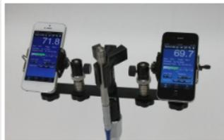
Figure 1. The SoundMeter app on the iPhone 5 (L) and iPhone 4S (R) compared to 1/2" Larson-Davis 2559 random incidence type 1 microphone (C).
